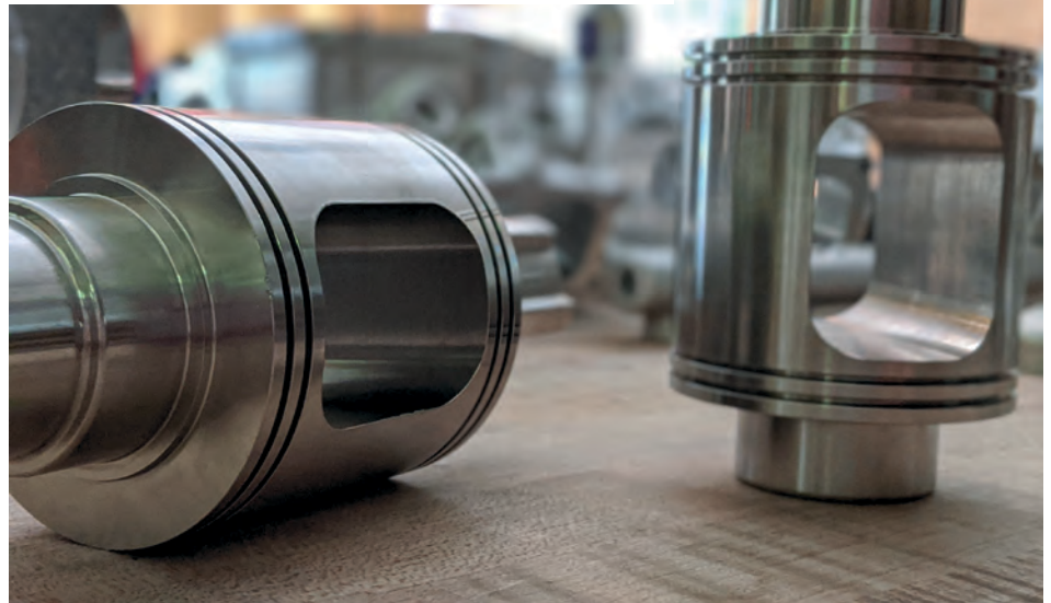
The rotary exhaust valves are machine-cut from stainless steel, and a seal is installed on each end of its cylindrical section
