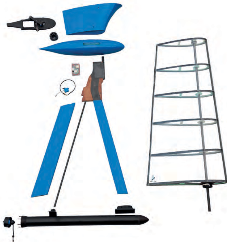
This exploded view shows the major components. Note the computer module in the centre and the sail regulation mechanism at the upper left
