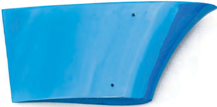
The upper float module is the part that pierces the surface. It is kept as small as practical to minimise wave-making drag
