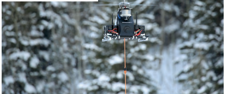
The E7500 UAV uses a coaxial rotor configuration, with flapping hinges and additional electric lateral-thrust motors for stable flight and carrying underslung payloads (Courtesy of FulcrumAir)
