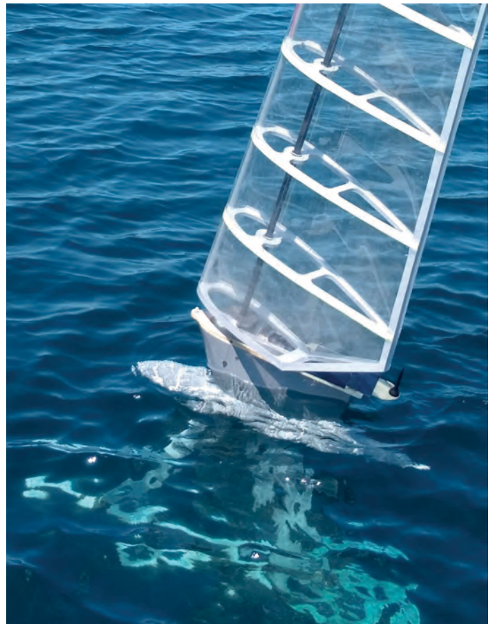
The ‘perturb and test’ autonomous sailing method is based on finding headings that maximise the ‘velocity made good’ towards the next waypoint without the need for direct wind measurement
