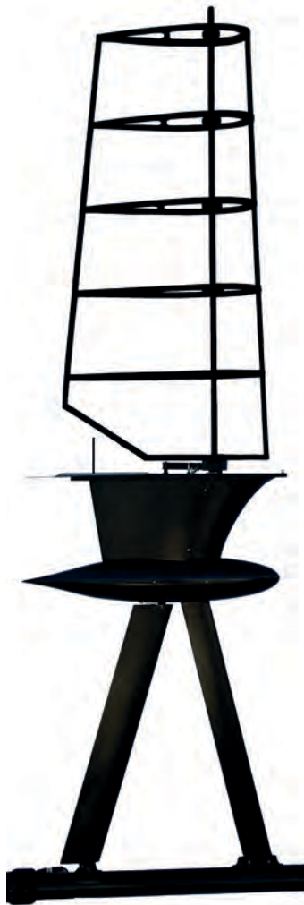
The Gen6 main hull has an interchangeable payload module in the nose. Above it are the keel, rudder post and rudder
