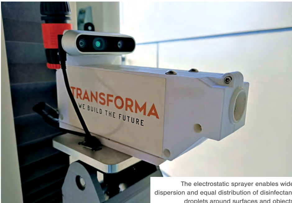
An Intel Realsense D435i depth camera is fitted on the nozzle, and embedded with AI from Hand Plus Robotics to recognise where to spray
