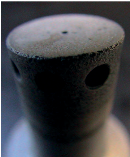
The original engine used a 'pepper pot' type of pre-combustion chamber; this has since been replaced with a chute-type pre-chamber on the Gen 2 WAM engines
