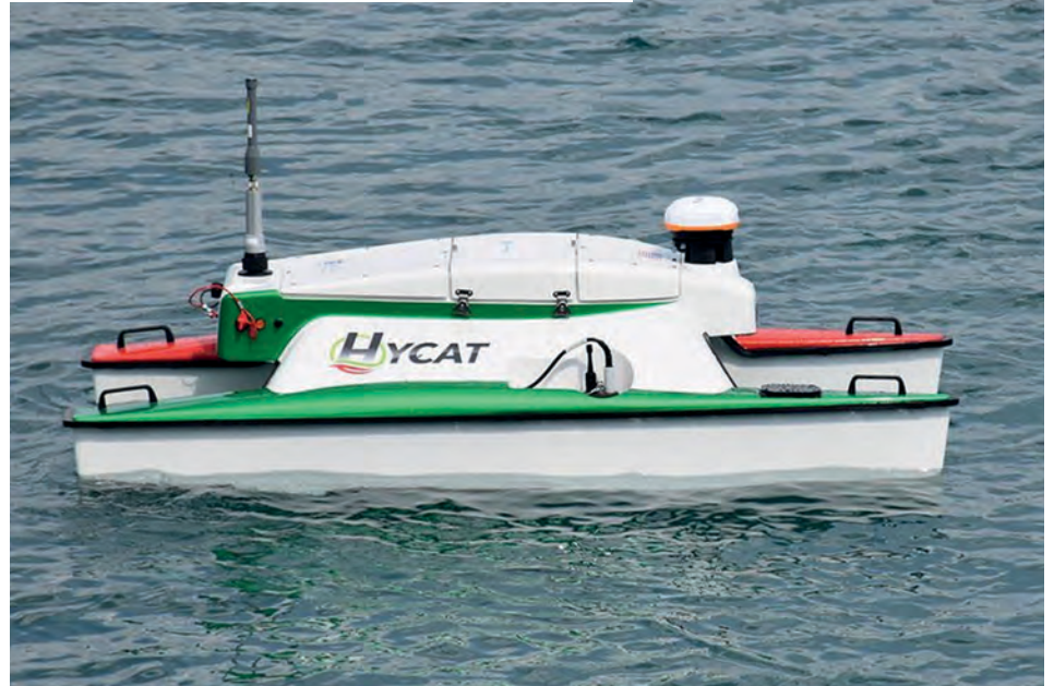
The HYCAT has been developed for water quality data acquisition. It uses control software closely integrated with survey software (Courtesy of SeaRobotics)
