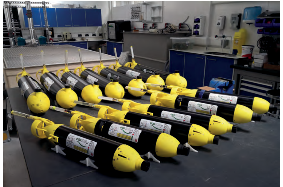
Production-standard ecoSUB \mu 5s (foreground) and m5s (behind). Note the multi-frequency comms and GNSS antenna on each – horizontal on the \mu 5s and upright on the m5s (Courtesy of ecoSUB Robotics)
