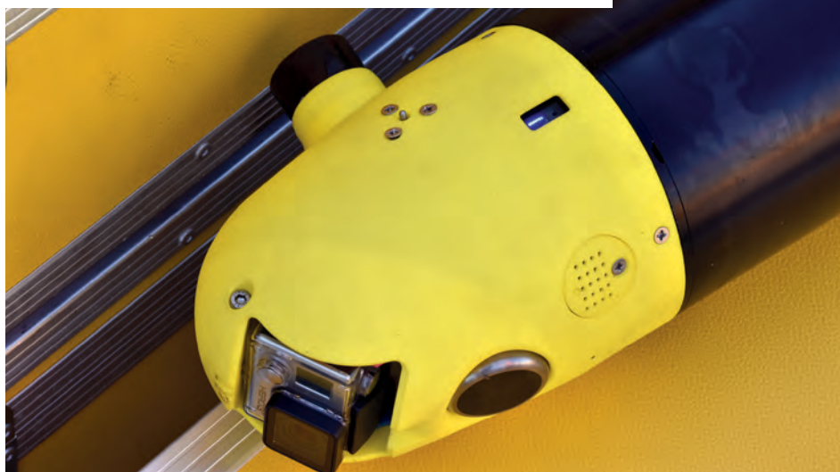
Bespoke nose cones for sensors such as this GoPro camera, acoustic modem and altimeter can be created easily using 3D printing, making integration of new sensors simpler (Courtesy of ecoSUB Robotics)
