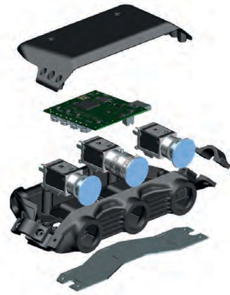
Exploded view of the camera sensor's architecture
