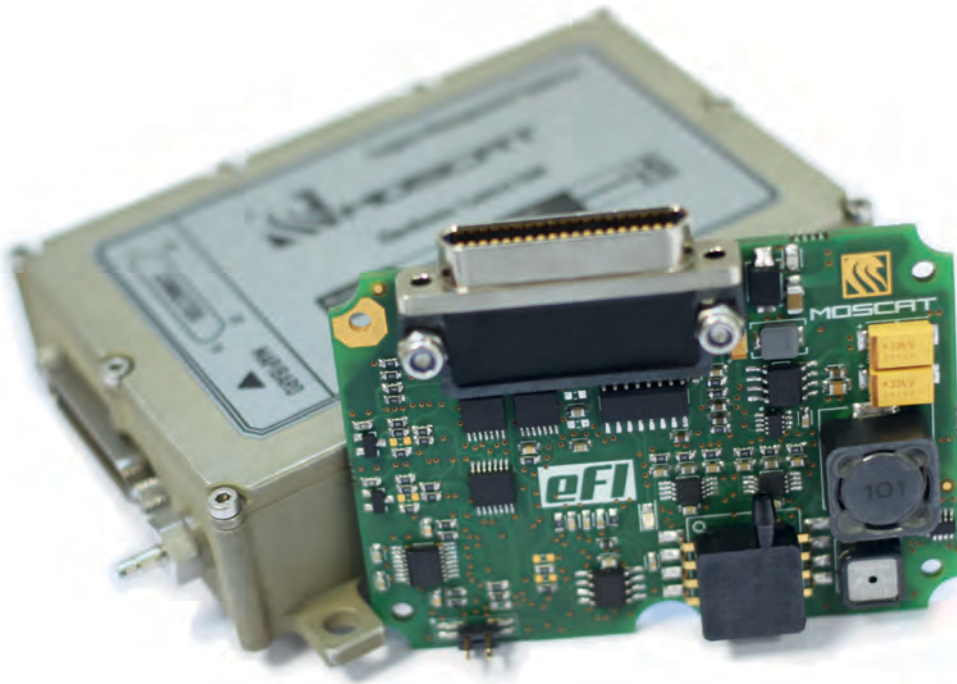
ECUs must handle a broad range of inputs and outputs, which is certain to widen as hybridisation and increasingly complex payload systems draw on engine power and torque generation (Courtesy of Moscat Ingenieria)
