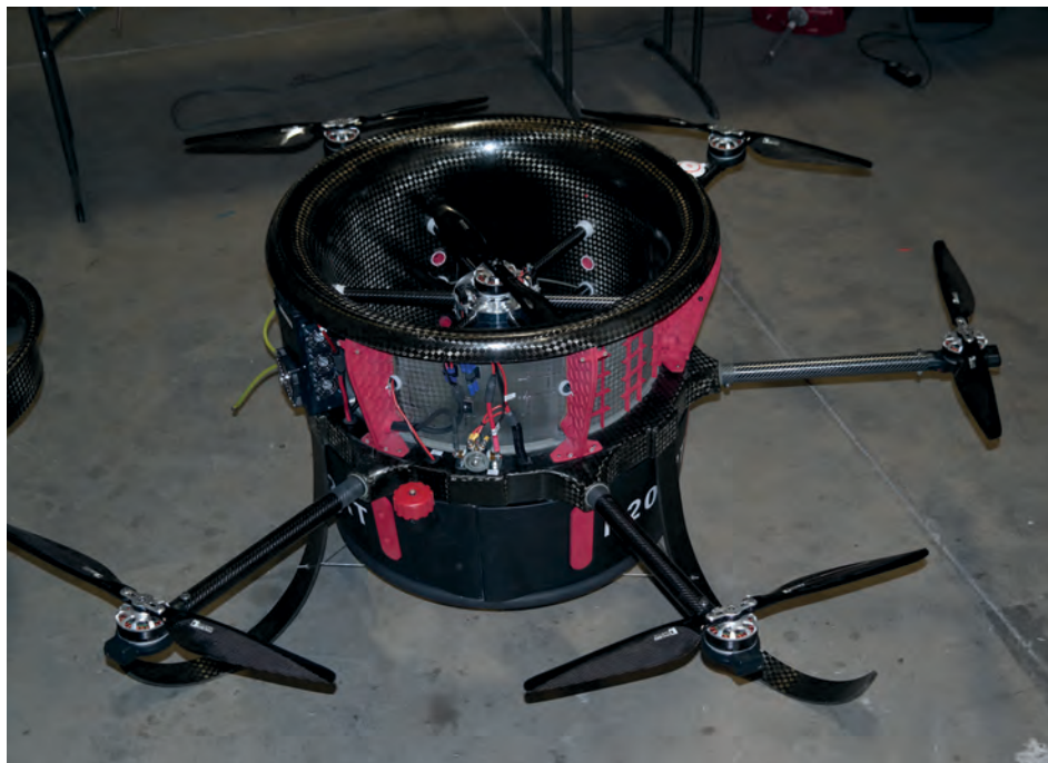
Like the external rotors, the one in the central duct is electrically driven, but it is controlled by the power management system rather than the flight control system (Courtesy of Reference Technologies)
