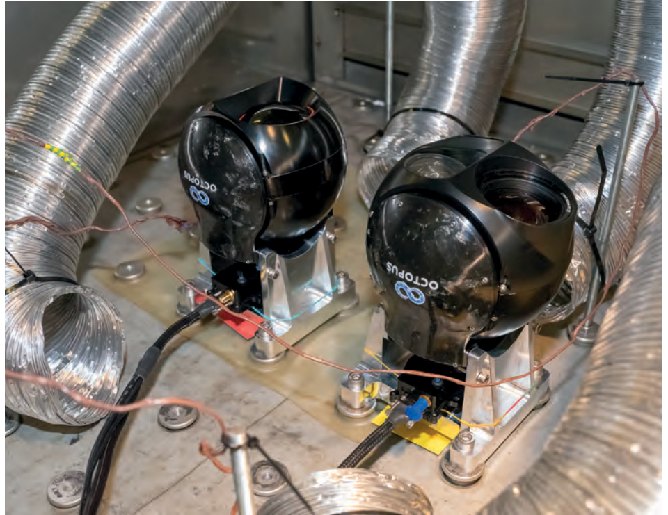
Highly accelerated stress screening can be used to unearth a gimbal's likeliest eventual point of failure, and correct it, before repeating the process for further testing and optimisation (Courtesy of UAV Factory)
