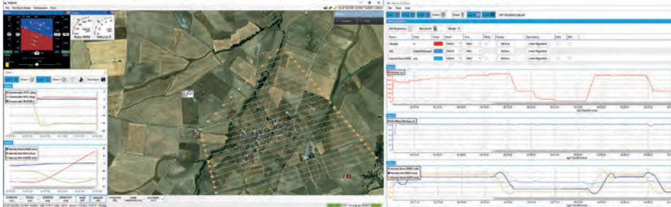
Performance monitoring is integrated into autopilot software to allow UAV operators to replay a flight with visibility of all the parameters (Courtesy of UAV Navigation)
