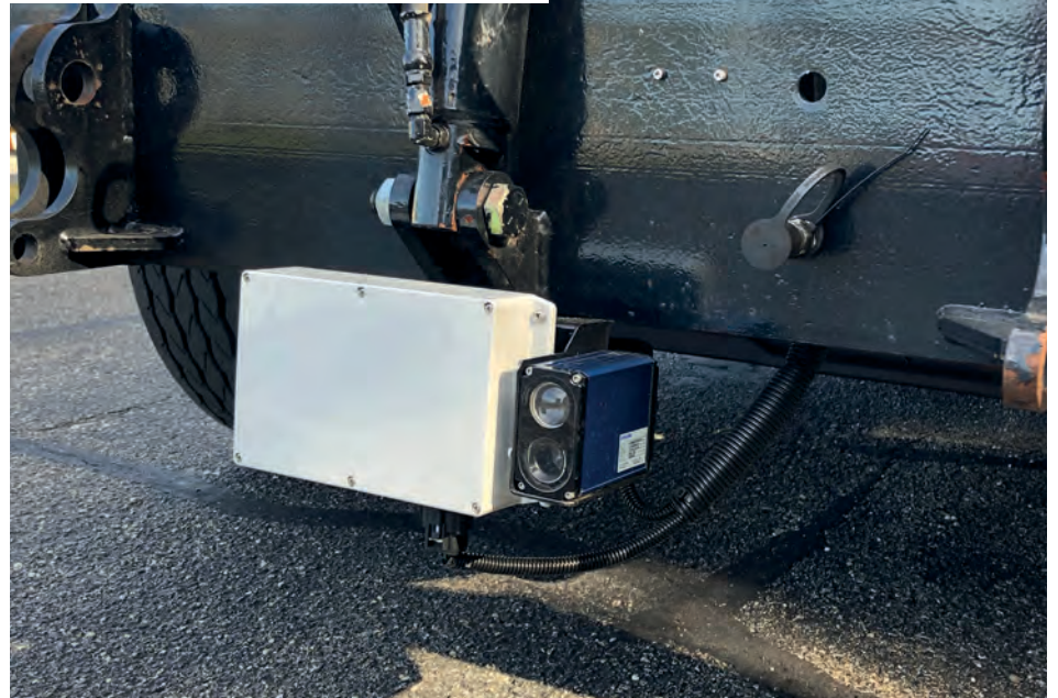
A Delphi electronically scanning radar is integrated at the front of the follower truck to provide the primary long-range obstacle detection
