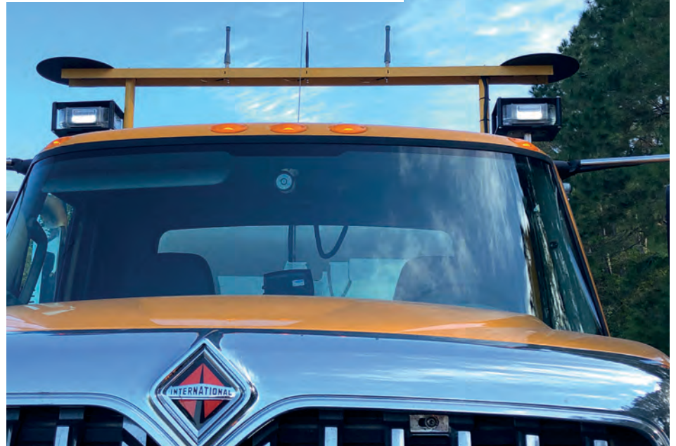
Cameras in the windshield of the follower vehicle and at the rear of the lead vehicle provide multiple vantage points of the work zone and the surrounding highway area
