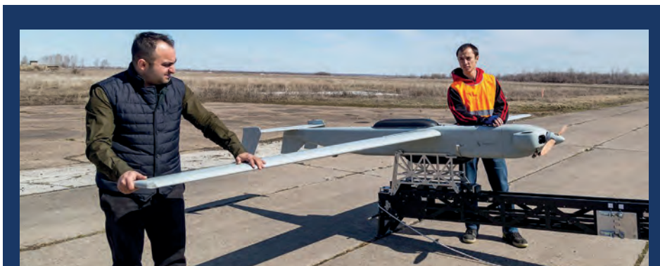
The Photon 601 uses machine vision to identify landmarks to navigate without the need for a GNSS satellite signal (Courtesy of University of Samara)
