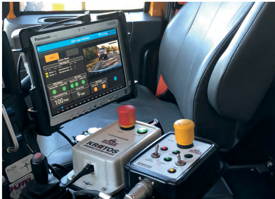
Panasonic's FZG1 ruggedised notebook provides the ATMA's user interface, which typically displays a number of indicator lights showing the status of crucial systems
