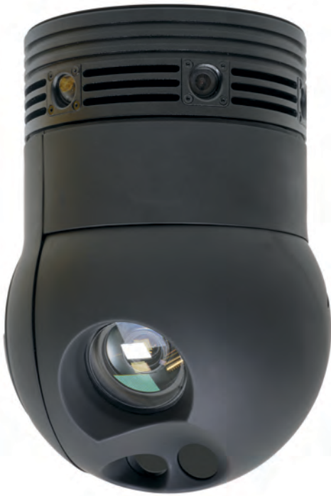
Cameras can be installed around the base of a gimbal to provide a 360° view for enhanced awareness and object detection (Courtesy of UAV Components)
