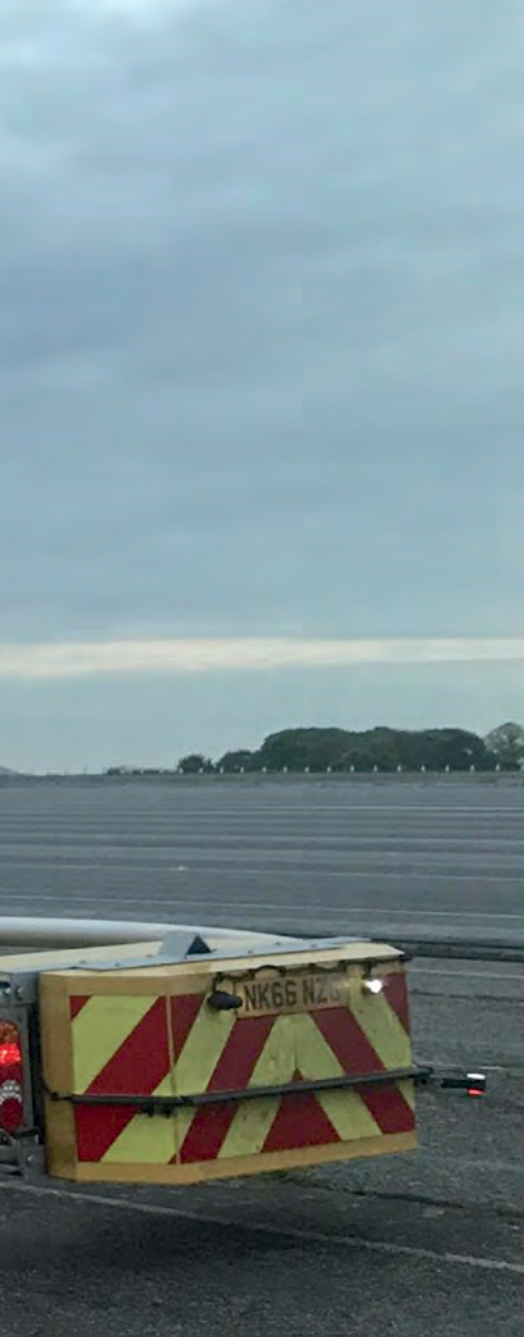
The ATMA system uses two trucks in a leader-follower arrangement, with the rear truck providing an autonomous crash barrier for what is typically a moving highway work zone (Photos courtesy of Kratos Defense)
