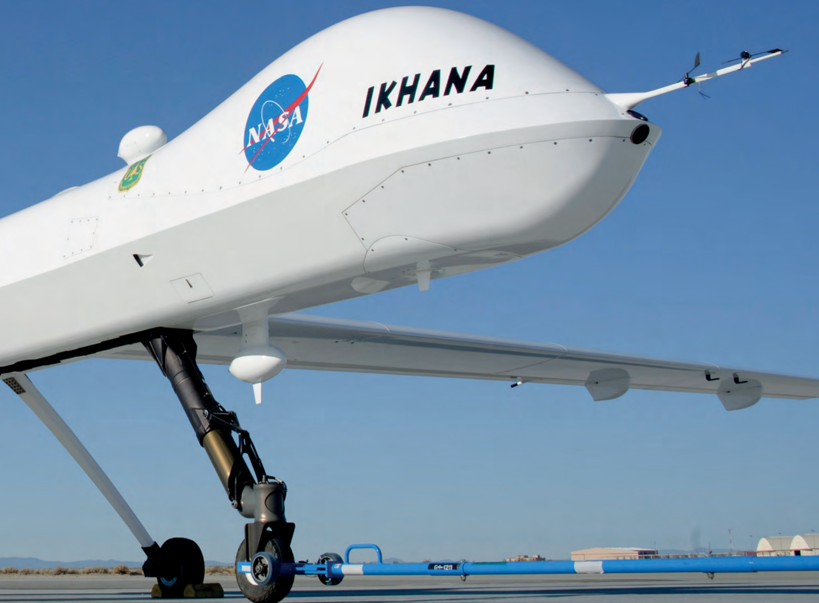
The Ikhana Predator B UAV is being used for sense and avoid trials linking onboard sensors to air traffic control and then notifying remote operators (Courtesy of NASA)
