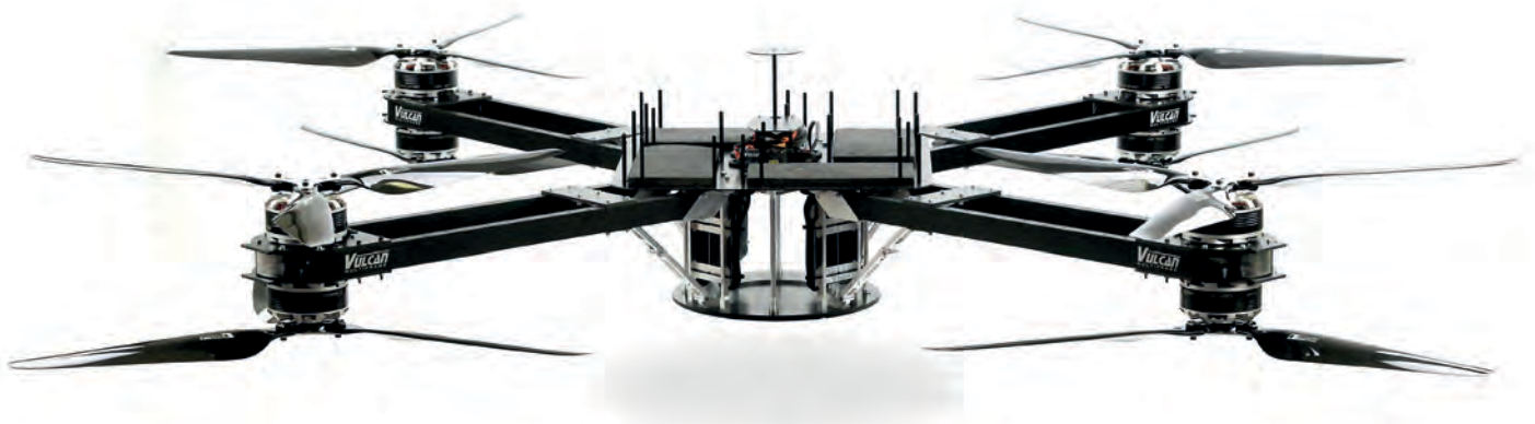
Vulcan UAV says its AirLift 2 will carry a 30 kg payload and have a flight time of up to 30 minutes
