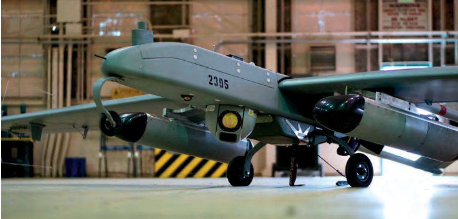
Pods with small radar systems are being installed on test systems for sense and avoid applications (Courtesy of IMSAR)
