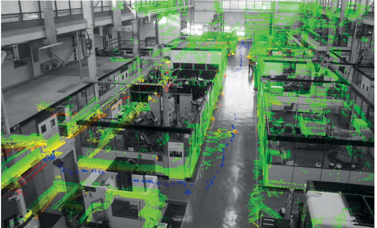
Laser rangefinder returns and hexacopter track visualisation from a project to develop a UAV that can safely fly through an unknown indoor environment using SLAM (Courtesy University of Warwick)
