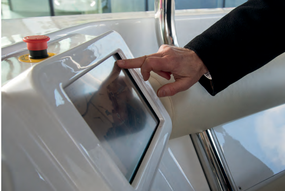
One control mechanism for driverless shuttles being tested in the GATEway project in Greenwich is passenger interaction via a touchscreen
